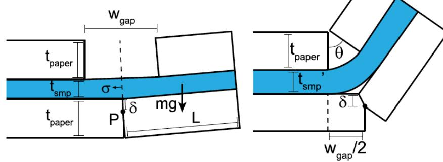
$$T = \frac{\sigma_a}{1 - \nu} W t_{\text{smp}} \left( \frac{t_{\text{smp}}}{2} + \delta \right)$$
